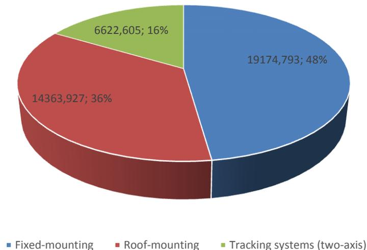
**Figure 11: Mounting installation description of PV systems in Cyprus up until the beginning of 2014**
