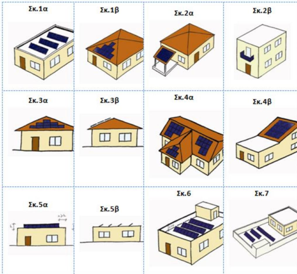
Figure 13: PV system installation guidelines of the Cypriot Circular 3/2008
